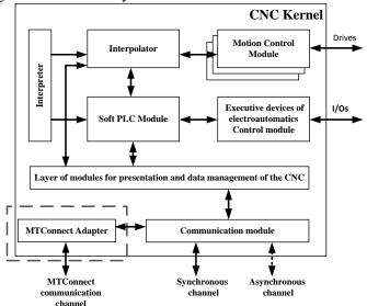
Figure 2. MTConnect Adapter in the kernel AxiOMA Control system.
