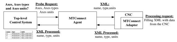
Figure 3. Example of the executing a Probe Request.
