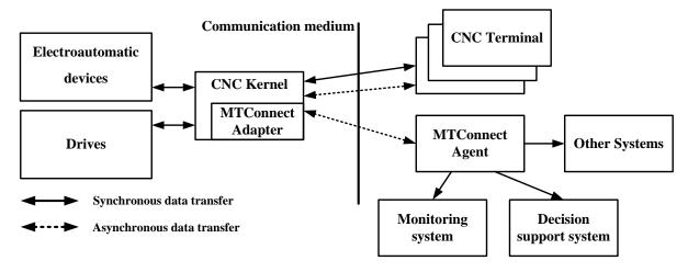
Figure 1. Interaction between the terminal and the kernel of the AxiOMA Control.
