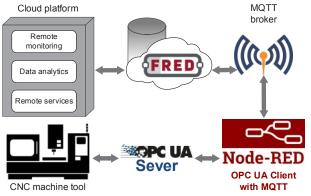
**Fig. 2.** Scheme of functioning of the test version of the digital shadow of the CNC system "AxiOMA Control".
